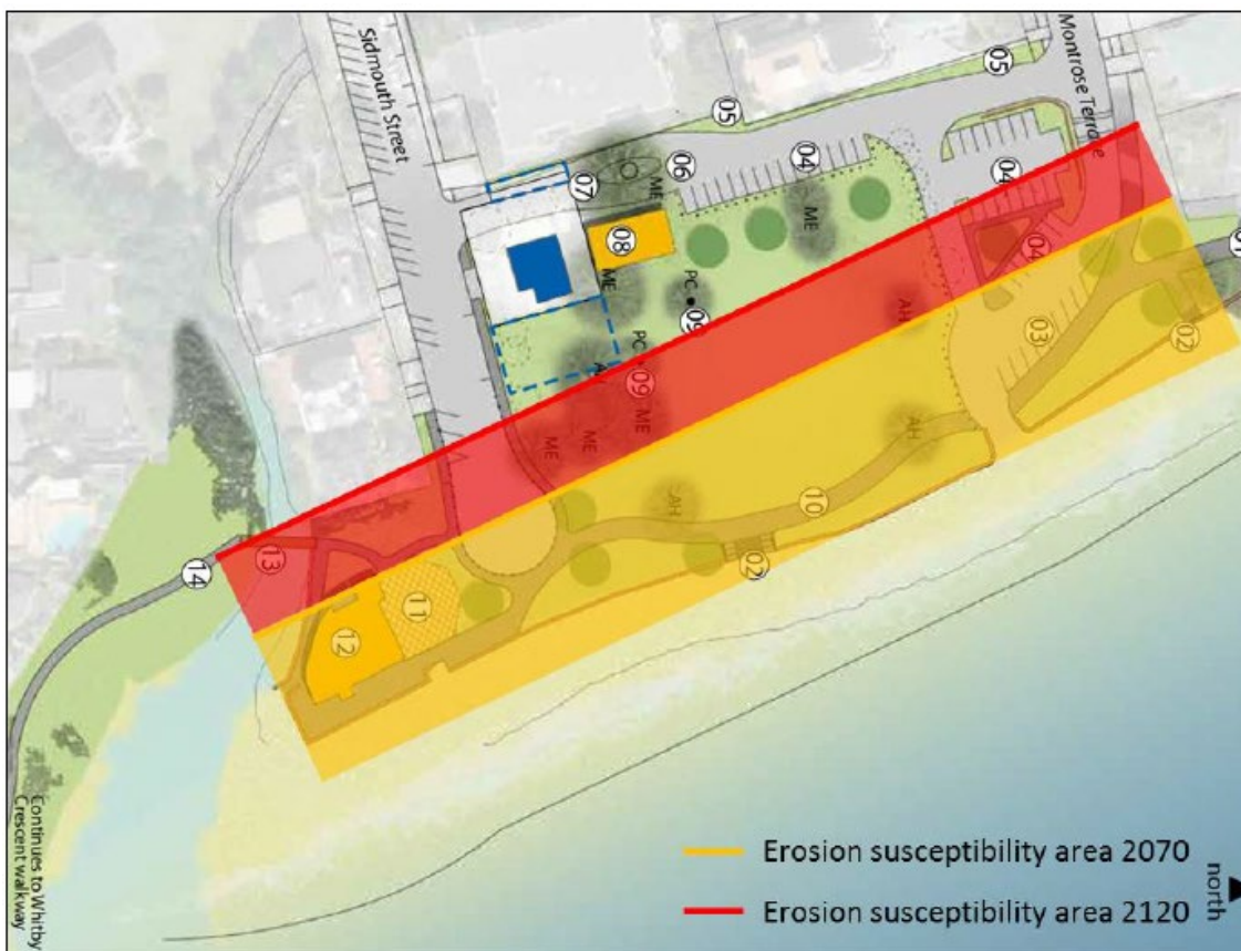
Figure 1 above – extract from the Shoreline Management Options Report 2022, showing the concept plan from the existing Reserve Management Plan, with erosion susceptibility layers for the next 50 and 100 years overlaid.
