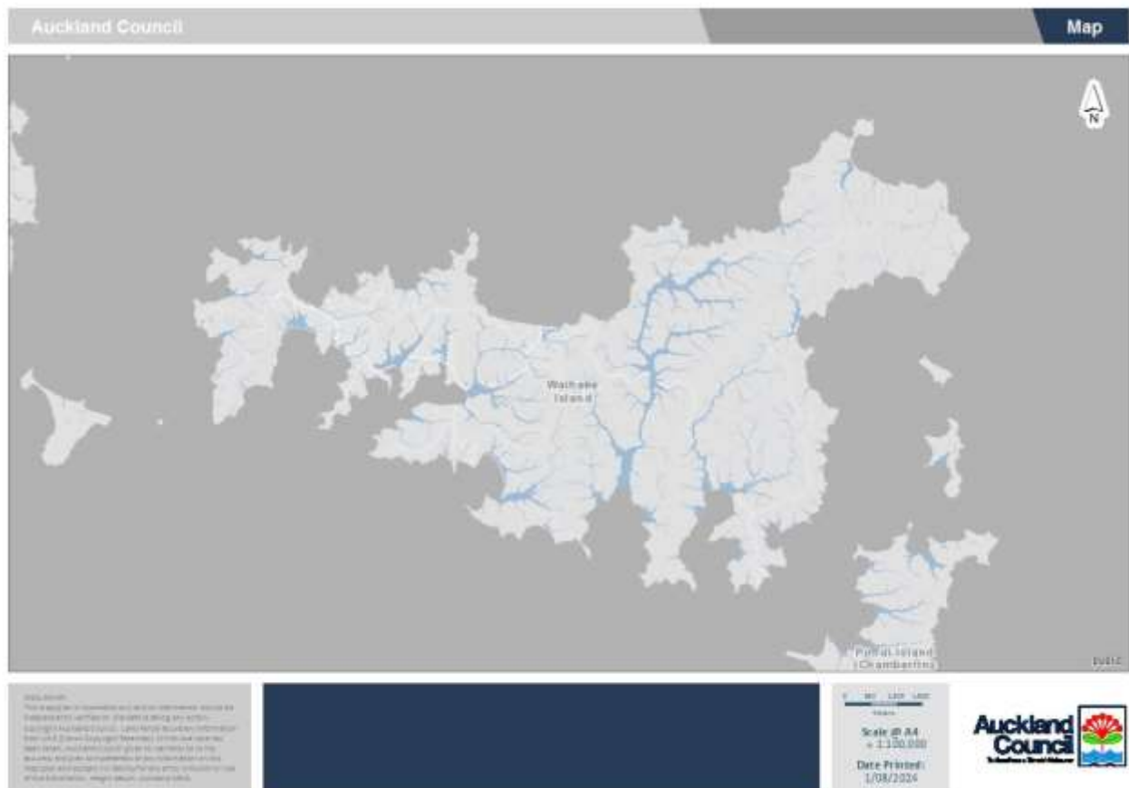
Figure 2- 4 Flood Plain areas 1% AEP (1 per cent annual exceedance probability) hazard, Auckland Council Flood viewer.
