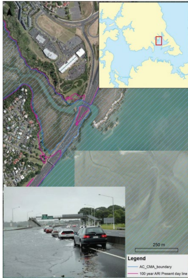
Figure 8-15: Verification of present-day 0.01 AEP (100-year ARI) storm-tide line against photograph of observed flooding on the Northern motorway during the 23 Jan 2011 storm-tide.
