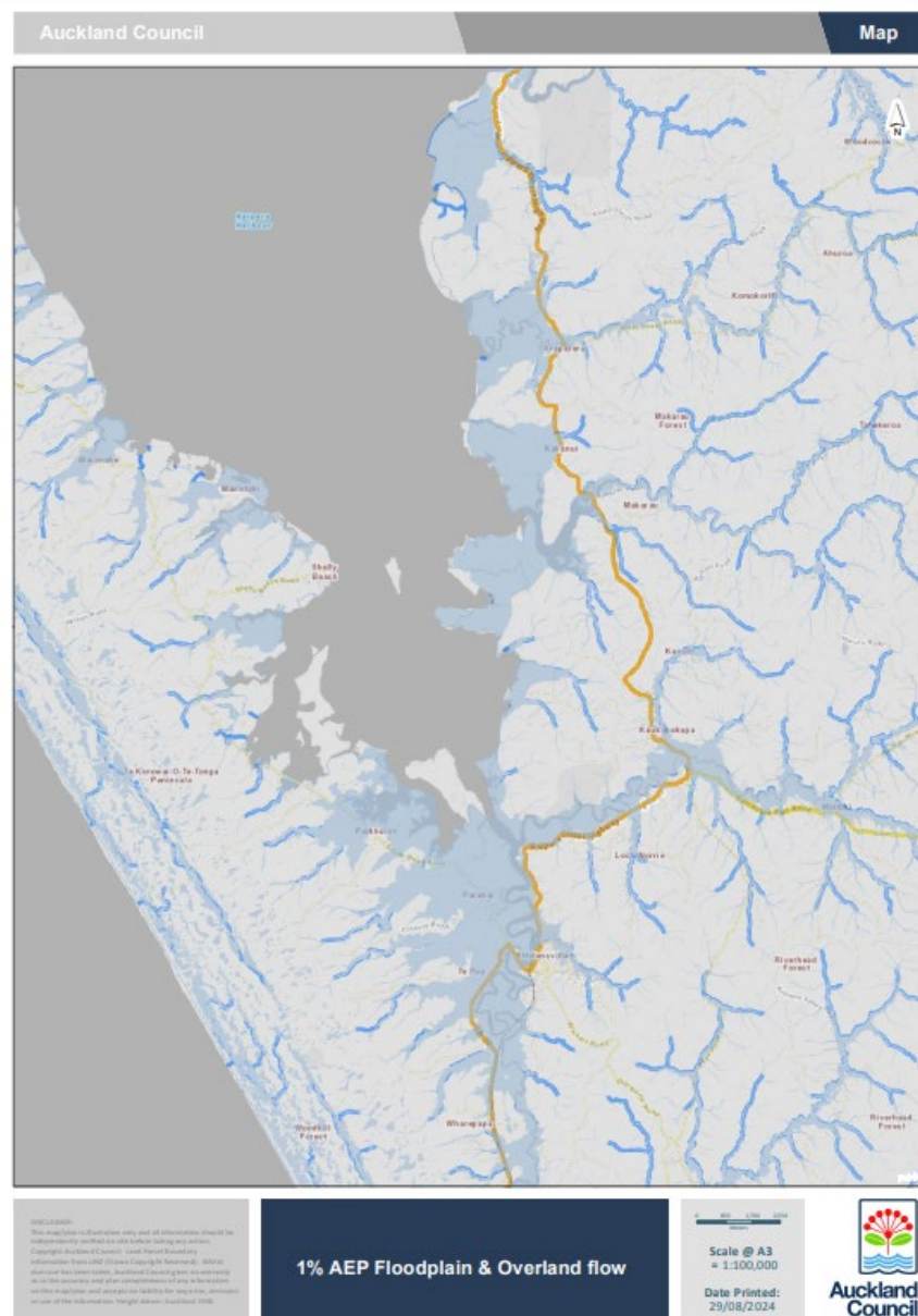
Figure 2- 6 Flood Plain areas 1% AEP hazard, area relevant to units 2-5 of the Kaipara Moana SAP area, Auckland Council Geomaps Flood viewer.
