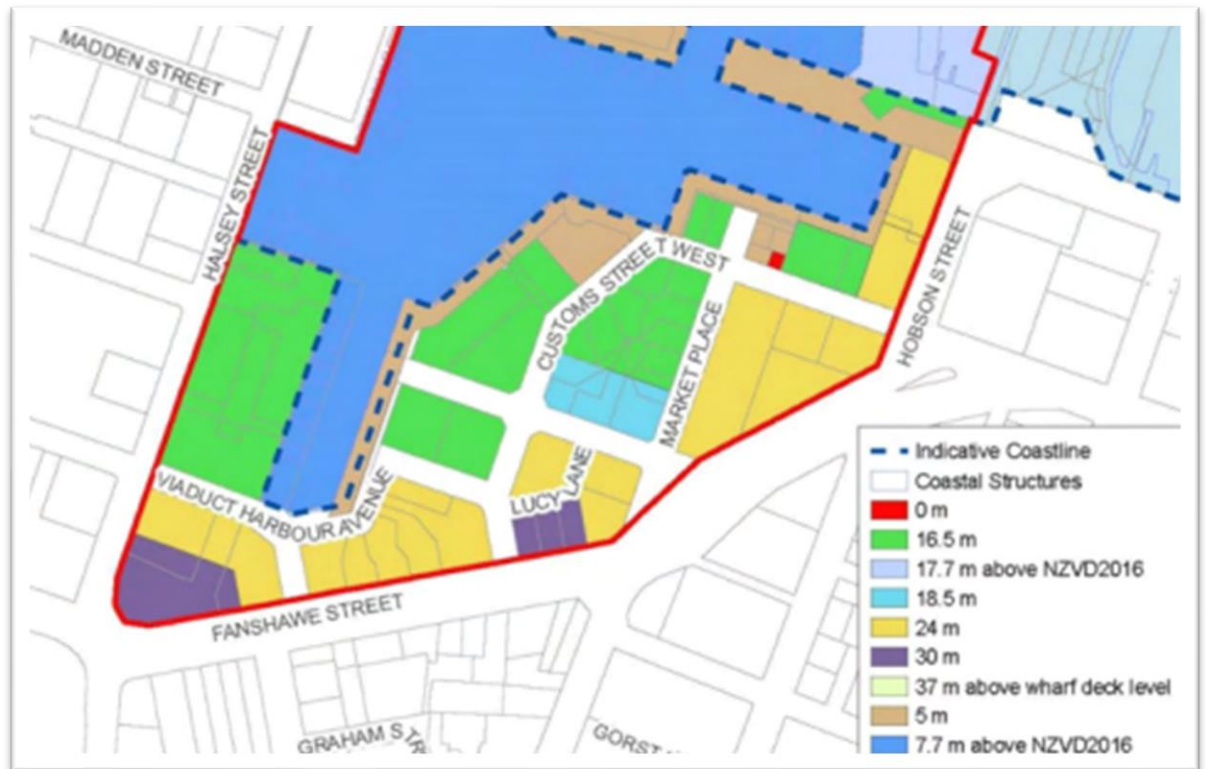
Figure 2: Viaduct Harbour building height controls
